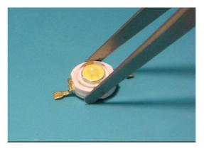
3、Manual mounting of LED onto MCPCB,Gently press the white plastic body or the lead
